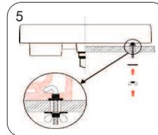
The face wash carefully propped up, slowly add the table after the hook bolt mounting holes aligned, and in accordance with the method shown in the table will wash fixed
