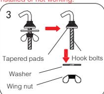
Remove the bolts from inside the product packaging washer and wing nut removed, leaving only the cone-shaped pads on the hook bolts.
