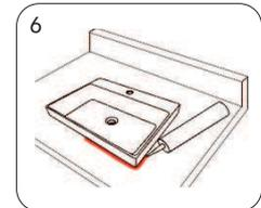
The maximum thickness of the mounting table is 35mm thick countertop will affect the strength of the installation, after installation, use a waterproof sealant around the edge of the wash basins and countertops in contact
