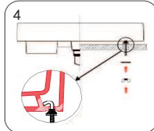
The hook bolts were placed around the mounting hole in the bottom of the wash basins on both sides and adjust the direction of the conical pad in the direction consistent with the mounting holes.
