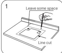
Depending on the installation location to install the sheet-like positioning wash pen wash basins installed along the edges of the sheet-like contour washbasin with mounting holes depicted in the table
